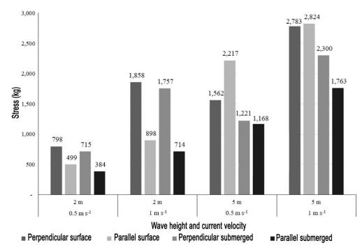
Figure 3. Stress on the mooring line under two operating conditions and different oceanographic variables.
