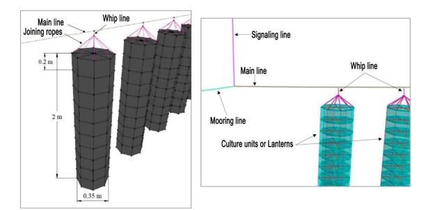
Figure 1. Components and dimensions of the culture unit (lantern).
