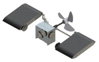
Figure 6. Complete undulation system with propeller, gear and hydrofoils.
