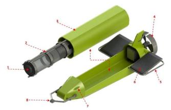
**Figure 14.** U-Tow IV. 1) Multiparameter probe, 2) mounting track, 3) transport box, 4) propellor guard, 5) hydrofoil guard, 6) hydrofoil, 7) inputs to the continuous flow of water, 8) tow hitch.
