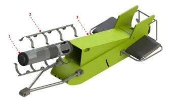
**Figure 11.** U-Tow III: Box for transport and mounting of the probe. 1) Multiparameter probe, 2) support and mounting track and 3) box for transport and housing of the probe.
