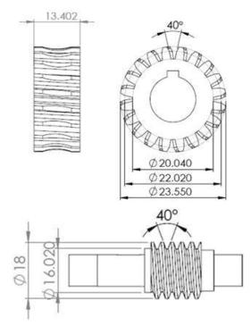
Figure 3. Cogged crown and auger screw, calculated according to Klebanov *et al.* (2008).
