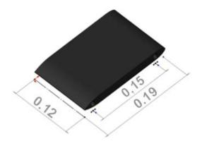
Figure 5. Isometric hydrofoil NACA 0012.
