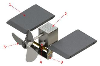
**Figure 15.** Undulating system with chassis for the U-Tow IV. 1) Hydrofoil, 2) gear, 3) chassis, 4) transmission of the gear to the undulators, 5) adjustable propeller pitch.
