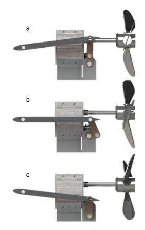
**Figure 7.** Movement of the hydrofoil with the arrangement of the two connecting rods. a) Maximum angle of attack, b) zero angle of attack, c) negative angle of attack.
