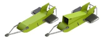
Figure 12. U-Tow III in closed and open views.
