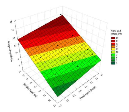
Figure 1. Wing-end spread of trawl nets according to the headrope length and the trawl speed.
