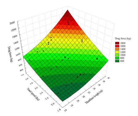
Figure 2. Trawl nets hydrodynamic resistance according to headrope length and trawl speed. The drag force corresponds to a simulation of an independent net.
